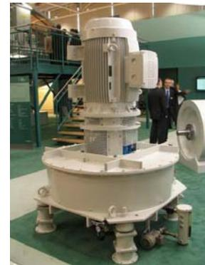
Fig. 4. Flywheel Energy Storage System (ENERCON, 200 kW, 5 kWh. Thanks to PEGE).
