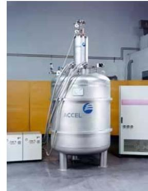
Fig. 3. SMES (200 kW, 2 MJ. Thanks to ACCEL).
